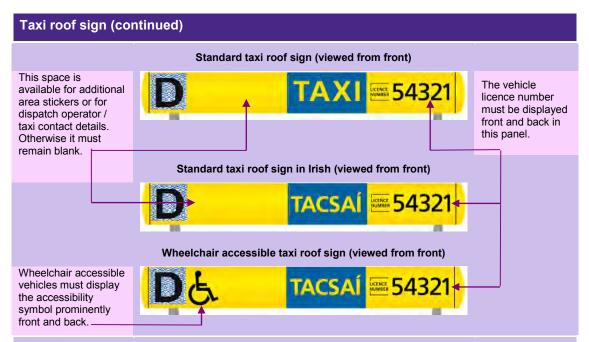
The roof sign must incorporate internal electric illumination that is switched on when the vehicle is available for hire and switched off when the vehicle is hired. Additional lights must not be attached to the regulation roof sign.
